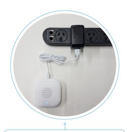
Connect the Gateway to a USB Power Adapter using a Micro USB Cable.
